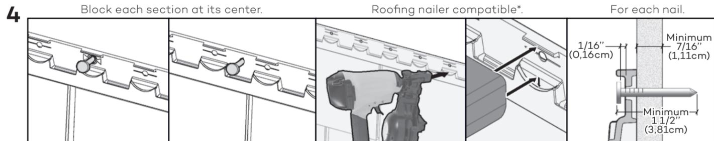
When installing a full section, nail in the center section, nail in its center. For each nail, leave a gap between nail head and section. When using a roofing nailer, adjust its tip at the highest position and the air pressure according to the substrate in order to leave the required gap.
