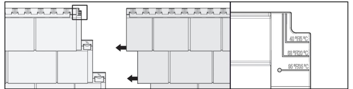
Below 40°F(5°C), position the section slightly right (1/16"(0,16cm)) of the 40°F(5°C) temperature line.
