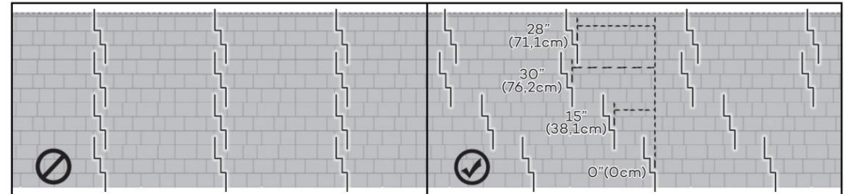
Alternate the joints between rows. For a nicer look, we suggest alternating the cutting distance of the first section of every row from 0"(0cm) - 15"(38,1cm) - 30"(76,2cm) - 28"(71,1cm).
